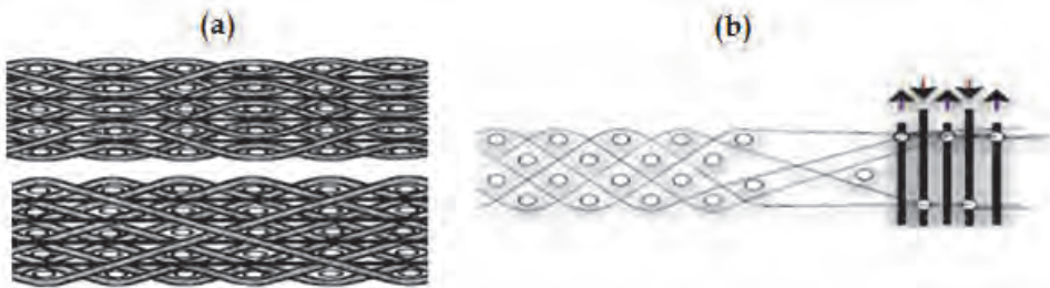
Fig. 9. 3D angle interlock fabrics (a) and schematic view of 3D weaving loom (b) (Khokar, 2001).
