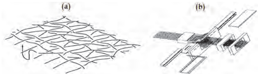
Fig. 15. Four layers multiaxis woven fabric (a) and narrow weaving loom (b) (Bryn et al., 2004).
